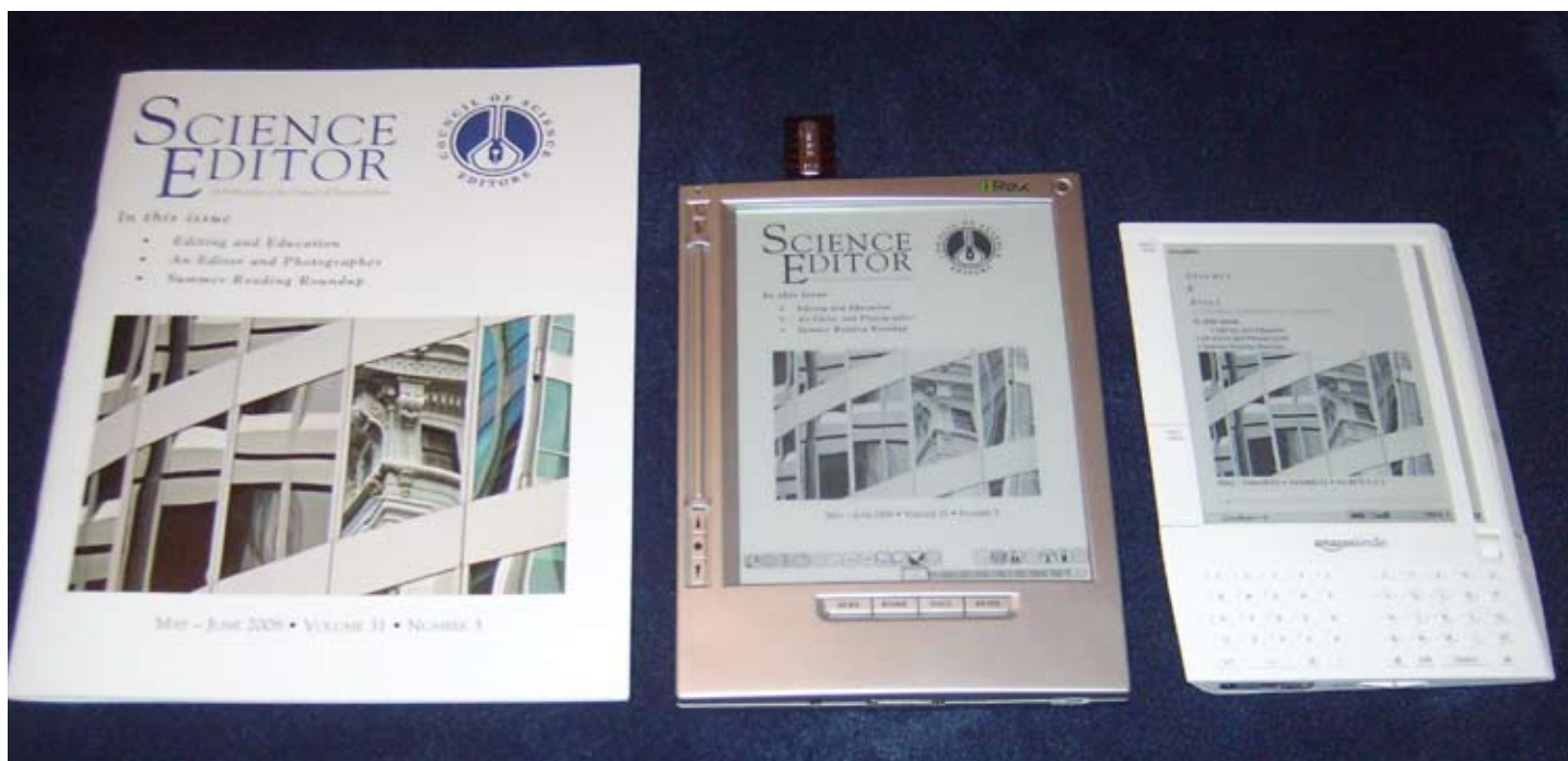
A printed issue of Science Editor as compared with the issue's pre-production PDF file displayed on the IREX Iliad and the Amazon Kindle. The photo shows some of the difficulties of viewing a PDF file on these e-book readers: decreased font size on the Iliad (although one can magnify portions of the page) and formatting problems on the Kindle.
